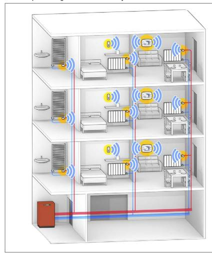
The controller receives the signal from the temperature sensor to establish the presence of heating demand in the zone in question on the basis of the programming. The valves located in the zone in question are adjusted accordingly.
