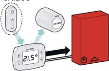
The temperature sensor is optional in that the electronic control head is already equipped with a built-in temperature sensor. Use of the sensor is recommended in the case of installation in conditions that could impair correct temperature readings. E.g., under deep shelves, as shown in the figure.
