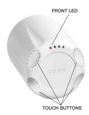
Electronic control heads code 210510 mounted to the valve of each radiator are indispensable to manage heating system zones. Modulating the flow rate of the thermal medium the control heads regulate the ambient temperature in accordance with the selected comfort level. The controller and electronic control head communicate every 10 minutes (20 minutes in summer mode) to maximise battery life.
