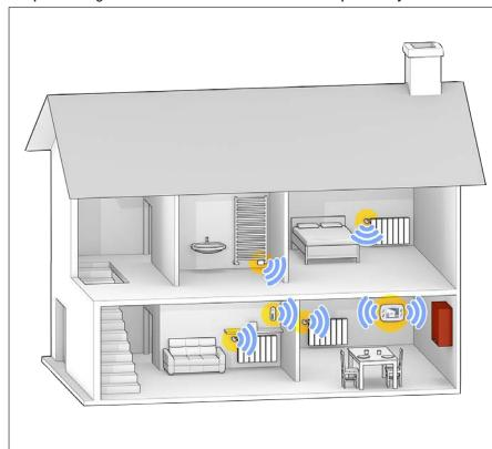
The controller receives the signal from the temperature sensor to establish the presence of heating demand in the zone in question on the basis of the programming. The valves located in the zone in question are adjusted accordingly. The boiler is started by means of the specific relay output in the presence of a heating demand from at least one of the zones.
