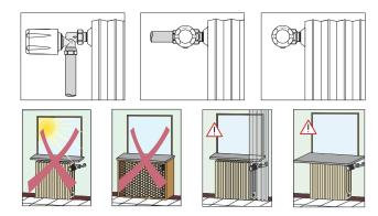
We recommend installing the chrono-thermostatic control heads in a horizontal position. Vertical positioning impairs correct temperature reading with consequent loss of accuracy in ambient temperature regulation.
