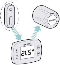
The temperature sensor is optional in that the electronic control head is already equipped with a built-in temperature sensor. Use of the sensor is recommended in the case of installation in conditions that could impair correct temperature readings. E.g., under deep shelves, as shown in the figure.
